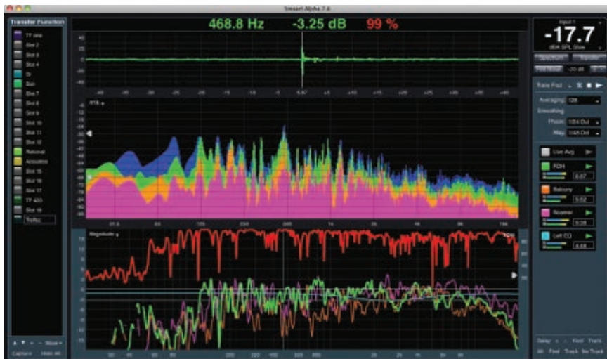
◀ FIGURE 1: Top Pane – Live IR; Middle Pane – 4x Live RTA; Bottom Pane – 4x Live Transfer Function.
